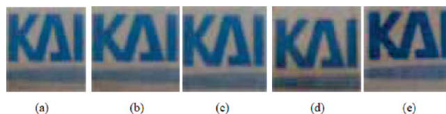
Figure 4. Films of (a) pure poly(methyl methacrylate) (PMMA) and (b–e) PMMA/acid-treated multiwalled carbon nanotube (c-MWNT) composites with different c-MWNT contents [(b) 1.8, (c) 4.5, (d) 9.8, and (e) 15.0 wt %].
